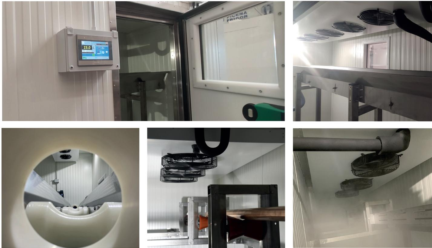
Refrigerators to be inserted along the production line of reinforced rubber hoses by spiraling on a rigid mandrel. They are designed with different lengths to be inserted along the production line so that the substrate reaches the spiraling machine with the correct temperature.
