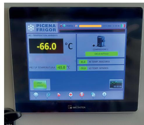
Machines used for laboratory tests such as that of flexibility and stiffness of hydraulic hoses at low temperatures down to  $-80^{\circ}\text{C}$ .
